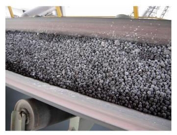
DRI **(B)**: а highly porous, black/grey metallic material formed by the reduction (removal of oxygen) of iron oxide at temperatures below the fusion point of iron. Cold-moulded briquettes are defined as those which have been moulded at a temperature less than 650°C or which have a density of less than 5,000 kg/m<sup>3</sup>. Fines and small particles under 6.35 mm in size shall not exceed 5% by weight.
