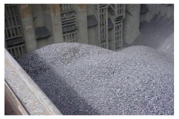
DRI (A): a metallic grey material, moulded in a briquette form, emanating from a densification process whereby the DRI feed material is moulded at a temperature greater than 650°C and has a density greater than 5,000 kg/m<sup>3</sup>. Fines and small particles (under 6.35 mm) shall not exceed 5% by weight. A loading requirement for DRI (A) is that moisture content shall be <1%.
